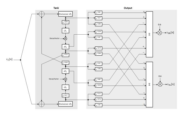
The following description tracks the signal as it progresses through the top of the tank. The signal progression through the bottom of the tank follows the same pattern, with different delay specifications.
