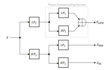
The phase-compensating section is equivalent to an allpass filter.
