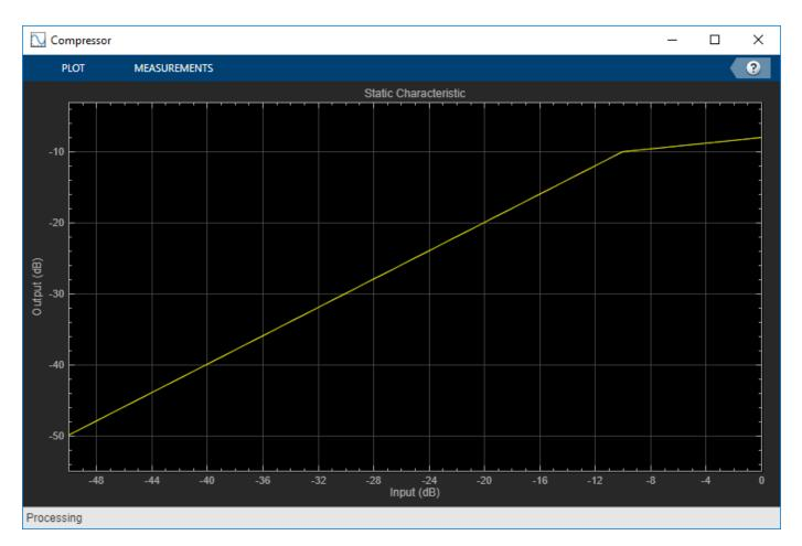
The static characteristic plot updates automatically if you modify a property of the object. dynamicRangeCompressor.Threshold = -30;
