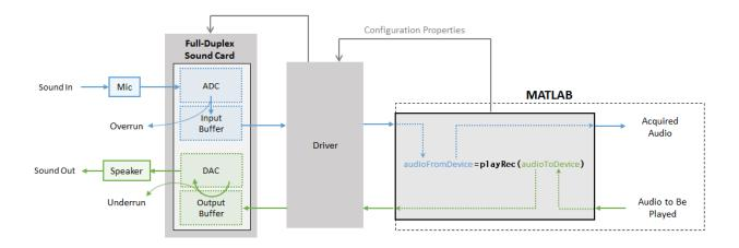
See "Audio I/O: Buffering, Latency, and Throughput" for a detailed explanation of the data flow.
