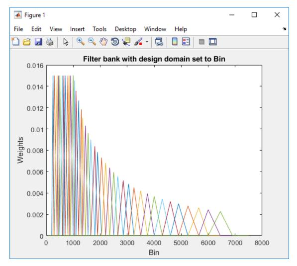
• Bin -- The band edge frequencies in Hz are converted to bins. The filter bank triangles are drawn symmetrically in bins.
