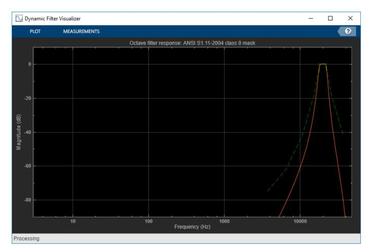
Another option to bring the octave filter design into compliance is to set the **Oversample** property to true. This designs and runs the filter at twice the specified **SampleRate** to reduce the effects of the bilinear transformation during the design stage.
