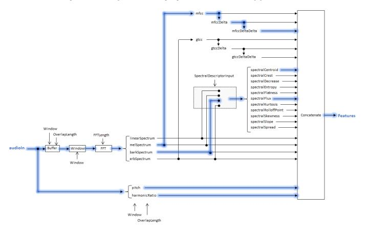
**Note** Because audioFeatureExtractor reuses intermediary representations, the features output from audioFeatureExtractor may not correspond with the default configuration of features output by corresponding individual feature extractors.
