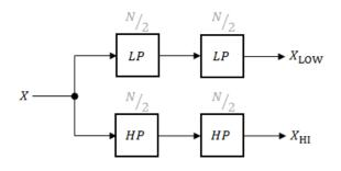
*LP* and *HP* are Butterworth filters of order N/2, where N is the order of the overall filter. The filters are implemented as direct-form II transposed second-order sections.
