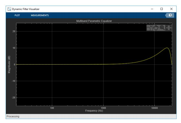
The equalizer band is warped.
