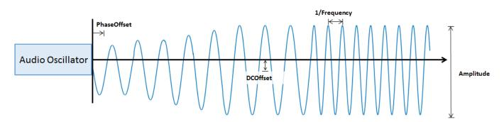
To generate tunable waveforms:
