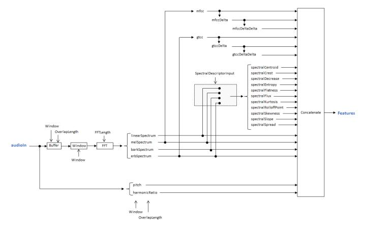
For example, to create an object that extracts the centroid of the Bark spectrum, the flux of the Bark spectrum, the pitch, the harmonic ratio, and the delta-delta of the MFCC, specify the audioFeatureExtractor as:
