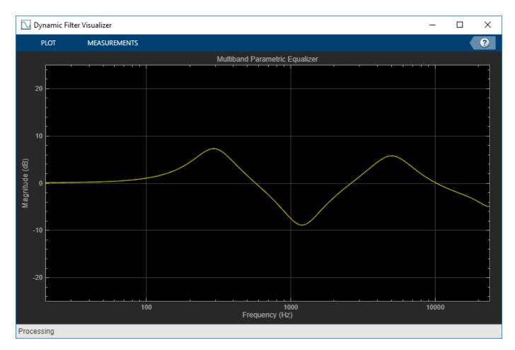
Play the equalized audio signal. Update the peak gains of your equalizer band to hear the effect of the equalizer and visualize the changing magnitude response.
