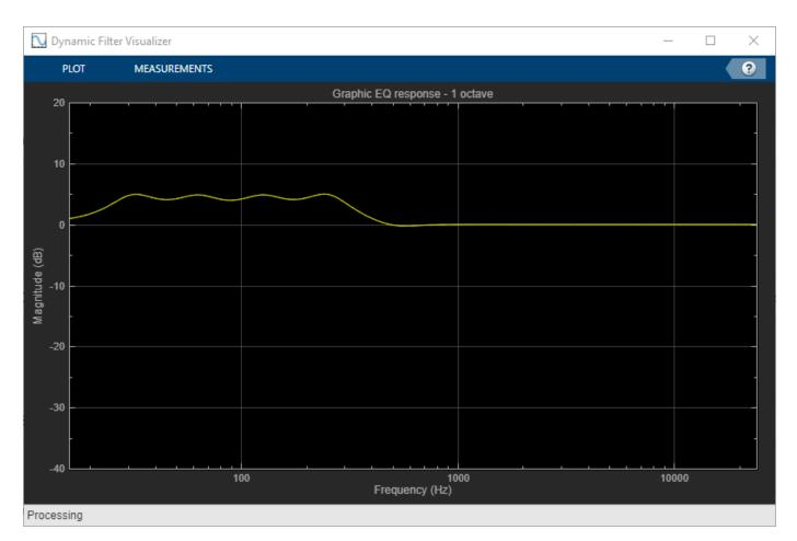
In an audio stream loop, read audio from a file, apply equalization, and then play the equalized audio through your audio device.
