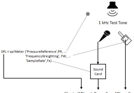
calibrate (SPL, micRecording, SPLreading)
