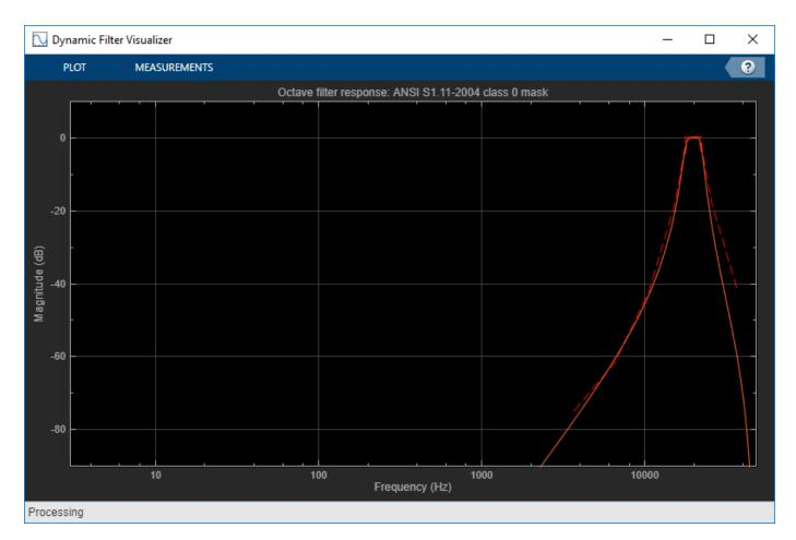
The red mask on the plot defines the bounds for the magnitude response of the filter. The magnitude response of this filter goes above the upper bound of the compliance mask around 6.6 kHz. One way to counter this is to increase the filter order so that the filter's rolloff is steeper.
