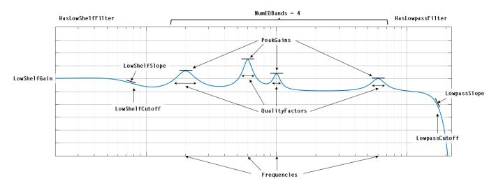
To implement a multiband parametric equalizer:
