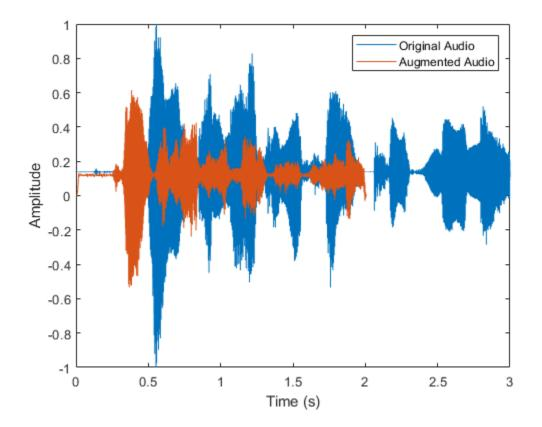
To partially compensate for the audible distortion and increase the fidelity of the augmentation algorithms, apply formant preservation to the shiftPitch algorithm, apply phase-locking to both algorithms, and change the cepstral order of the shiftPitch algorithm to 25. Listen to the processed audio.
