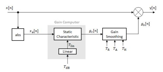
**1** The *N*-point signal, *x*[*n*], is converted to magnitude:
