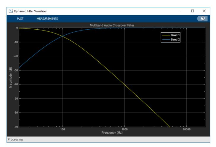
Call parameterTuner to open a UI to tune parameters of the crossover filter while streaming. parameterTuner(xFilt)
