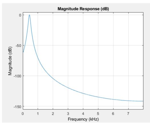
To specify the number of FFT points used to compute the frequency response, use the NFFT namevalue pair. Specify that the frequency response is calculated using a 8192-point FFT.
