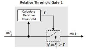
**a** The relative threshold,  $\Gamma$ , is computed:
