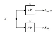
*LP* and *HP* are Butterworth filters of order *N*, implemented as direct-form II transposed second-order sections. The shared cutoff frequency used in their design corresponds to the crossover of the resulting bands.
