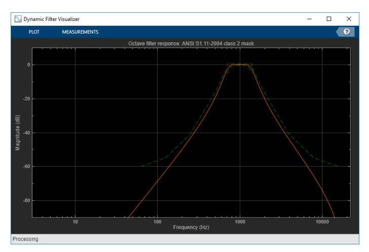
Analyze the filter using fvtool.
